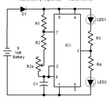
The basic operation of the circuit is fairly straight forward and I will it explain it here. When the power supply is first connected a current flow will pass through the resistors R2a, R2 and R1 allowing the
