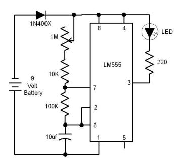
The resistance values are all in ohms. This circuit only uses 1 LED and the resistor is a smaller value for the LED, also the capacitor is a higher value so that more energy can be stored to flash the LED brightly and with a short duration then used in the alternating flasher circuit.
