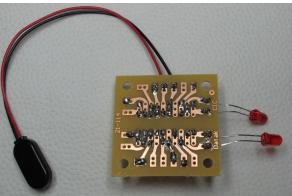
Now the assembling of the boards can be done. It is usually best to start with the items that need other parts fit around them first then move onto the balance of the components starting with the smallest and working your way to the largest. This is not a strict rule but I will give a list of steps that I would use for assembling this project.
