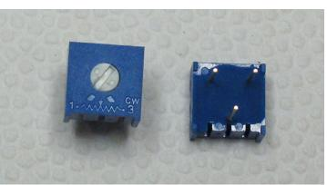
The **Potentiometer** used in this project is nothing more than a variable resistor. By using the center pin and one of the outside pins the dial can be rotated (about 300 degrees) which will vary the resistance value between 0 ohms and 1,000,000 ohms. Using this as R2a allows us to vary the flash rate for our LEDs.
