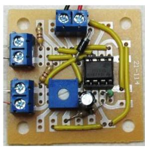
The LED's should start flashing at this point and you can adjust the potentiometer and you should see the flash rate change. If this is all working to your satisfaction you should now take a moment to label the terminals and add any other notes to the board using your fine tip marker.
